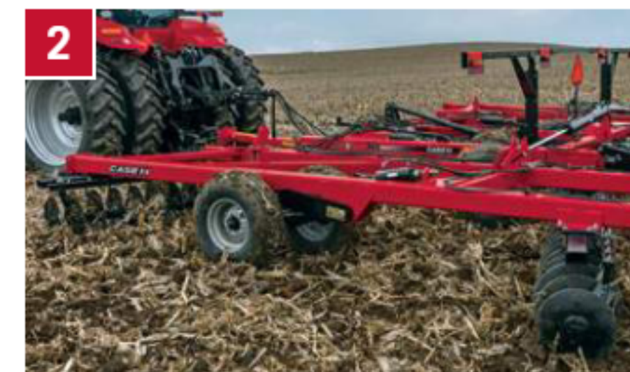
Disk gang depth: slice, cut and bury residue to the producer's desire.
