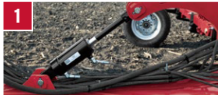
1 New hydraulic fore/aft control (Constant Level only): maintain consistent agronomic output
