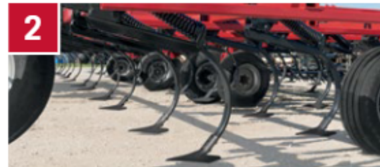
2 Shank depth: create an ideal seedbed surface and floor
