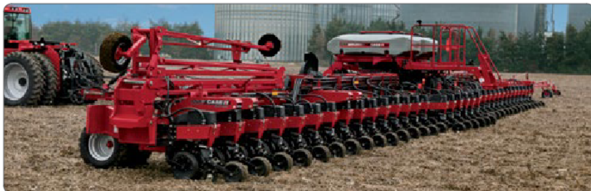
Case IH Early Riser® planters are designed with agronomics in mind and have multiple, patented features. The legendary Early Riser row unit has 12 unique features that all contribute to earlier, more uniform emergence, as well as an Advanced Seed Meter for accurate in-row spacing and population control.
