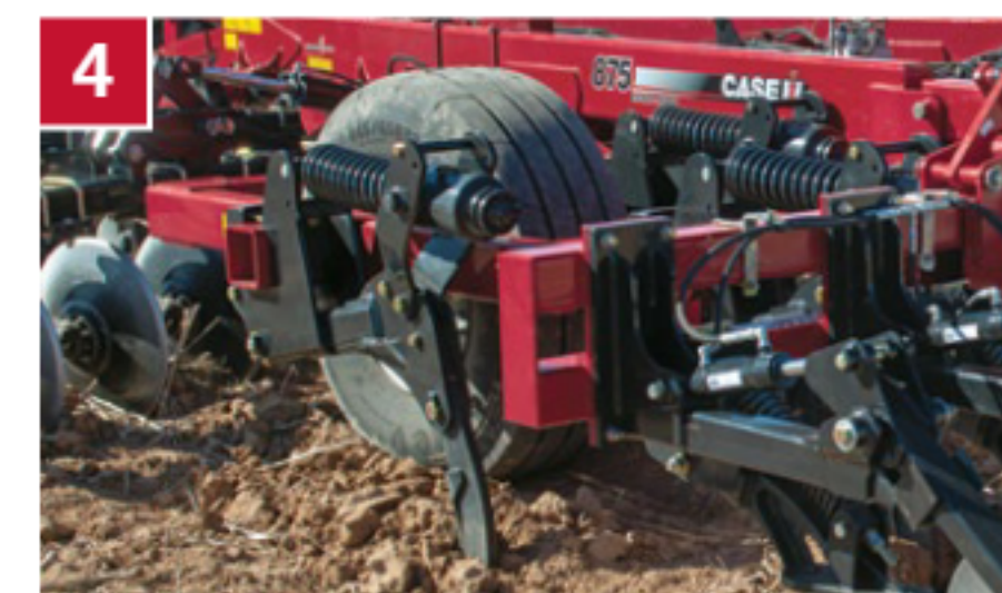
4 Shank depth: target the compaction layer
