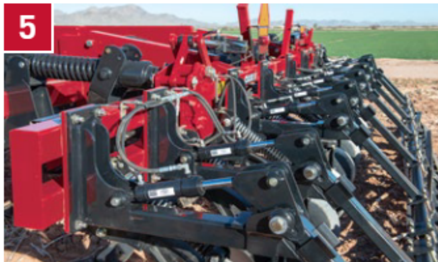
5 Crumbler pressure: achieve consistent clod sizing
