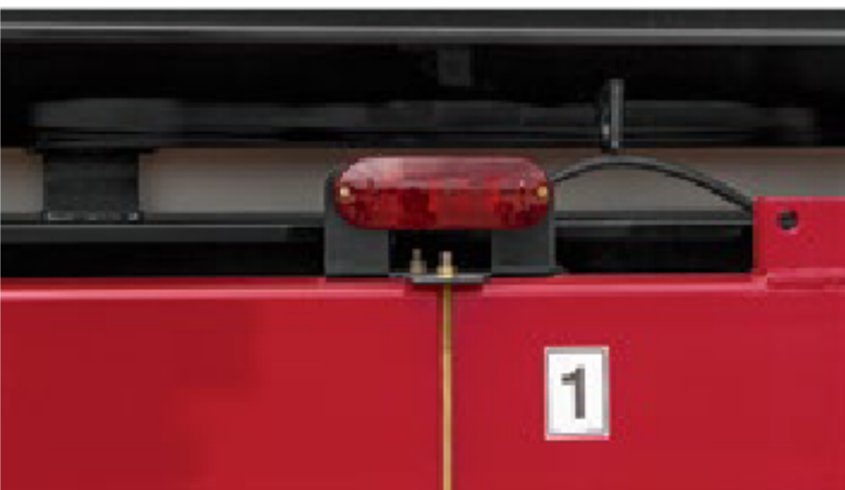
Tank full indicator lights.
