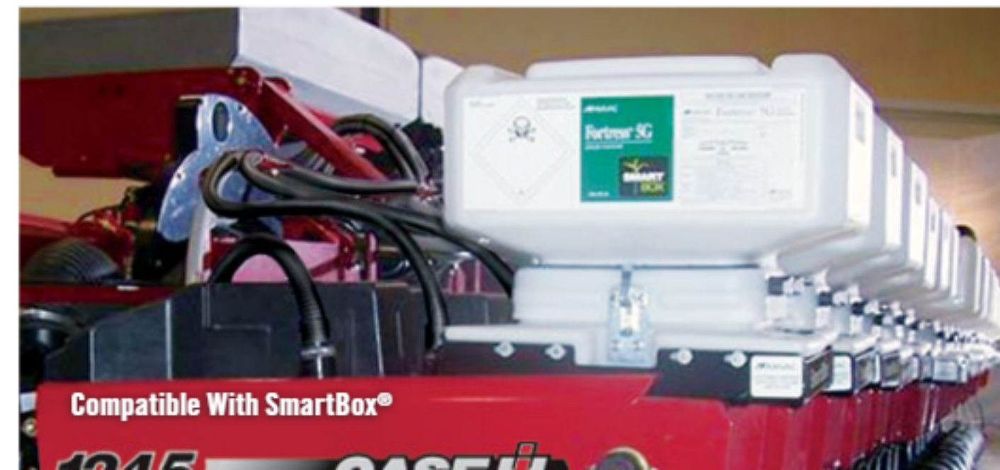
Granular Chemical Hopper
