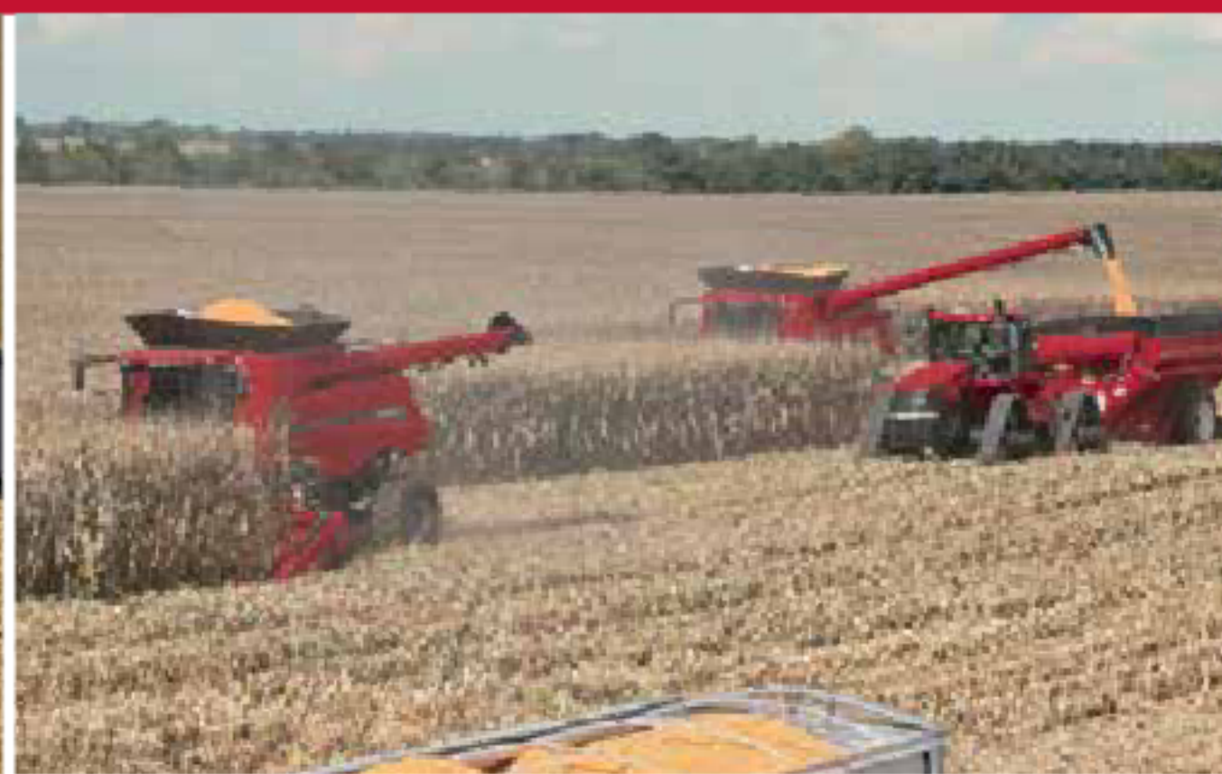
Exclusive Axial-Flow dual unloading system.
